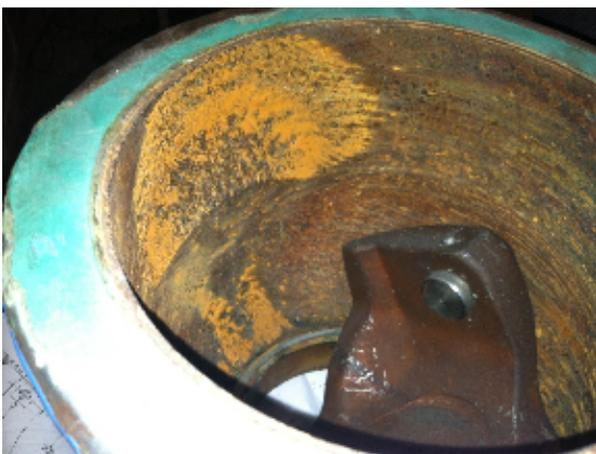
**Figure 1.** Severe pitting damage from cavitation resulted in a pinhole leak on the valve body of a V-notch Ball Valve used to regulate the cooling water flow to aluminum casting molds.
