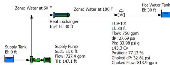
Figure 4. Control valve at 30 ft elevation.
