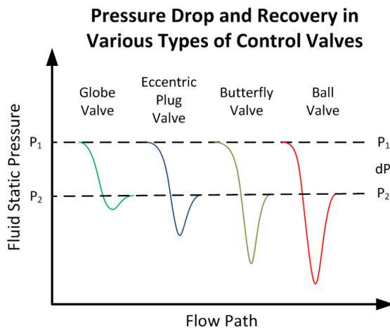
Figure 3. Pressure profile for various types of valves for a given pressure drop.
