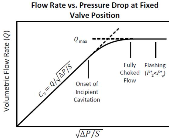
**Figure 2.** Graph of flow rate versus the square root of the pressure drop across the valve (courtesy of Crane Technical Paper TP-410).
