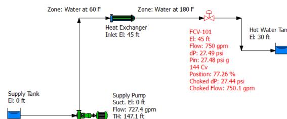
Because of the higher elevation, the inlet pressure of the control valve is lower (pressure head is converted to elevation head per the Bernoulli Theorem). This reduces the Choked dP and Choked Flow Rate according to Equations 2 and 3. Since the required dP across the control valve (27.49 psi) is greater than the Choked dP (27.44 psi), the valve would operate under choked flow conditions at 750 gpm.
