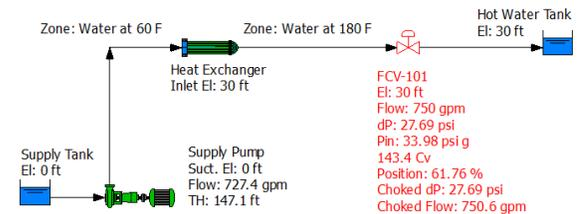
**Figure 7.** A different control valve with a lower  $F_L$  selected for the original system (valve at lower elevation with 180°F) results in choked flow.
