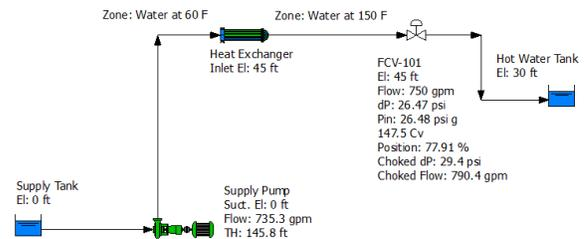
**Figure 6.** Colder water does not result in choked flow, even with the valve at the higher elevation.
