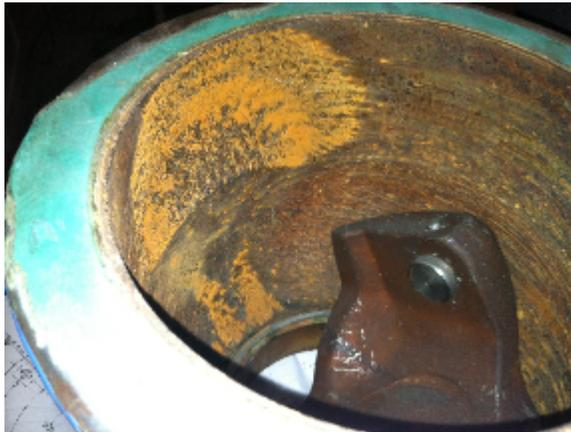
**Figure 1.** Severe pitting damage from cavitation resulted in a pinhole leak on the valve body of a V-notch Ball Valve used to regulate the cooling water flow to aluminum casting molds.
